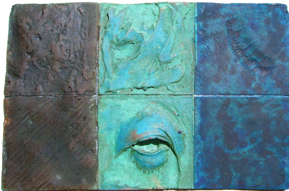
Copper cold cast resin with Mahogany, Light Green, and Vista Blue patinas (left to right).
