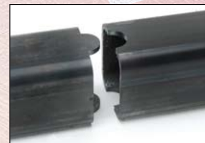
Tab & Slot cuts on 8" tube
